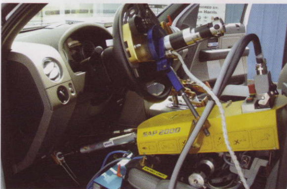
ABOVE LEFT: A driverless car equipped with ABD hardware awaits a test run
