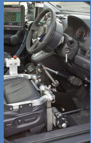
Driverless fish-hook test (above left), driverless misuse testing (bottom), on-seat DTS installed in a Honda (above right)
