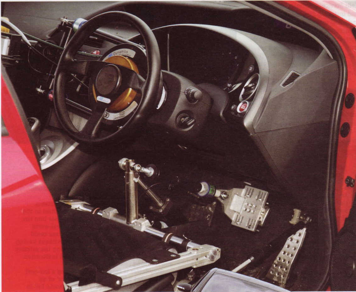
LEFT: ABD INSTALLATION IN A HONDA CIVIC. BELOW LEFT: DRIVERLESS SYSTEMS CAN REMOVE THE DANGER TO HUMANS FROM RISKY MANEUVERS
